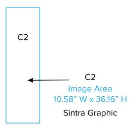
Panels 'A' & 'B' Note: 1" Hook Velcro on Back perimeter of Graphic Panels 'C1' & 'C2' Note: 1/4" of graphic perimeter is hidden by extrusion
